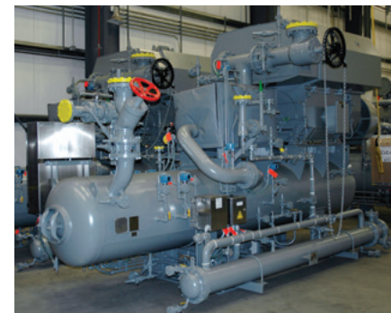
Ammonia BOG compressor package Model 565GL; 872 HP
