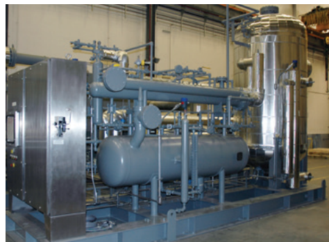
Ammonia condensing unit Model 1435GL; 1,750 HP
