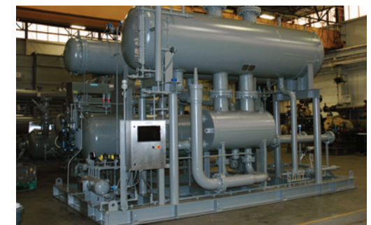
HTF chilling system
